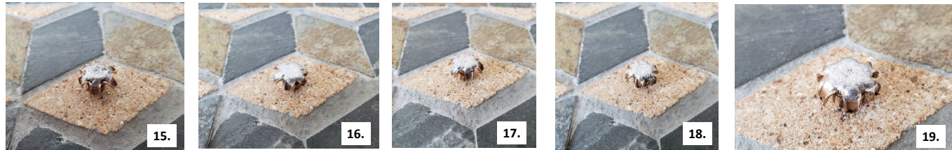
15. Federal Punch 30SC, 103gr JHP, 4-inch test barrel 16. Federal Punch 30SC, 103gr JHP, 4-inch test barrel 17. Federal Punch 30SC, 103gr JHP, 4-inch test barrel 18. Federal Punch 30SC, 103gr JHP, 4-inch test barrel 19. Federal Punch 30SC, 103gr JHP, 4-inch test barrel
